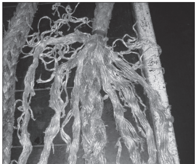
Figure 14: Tug D pendant (cut strands).
