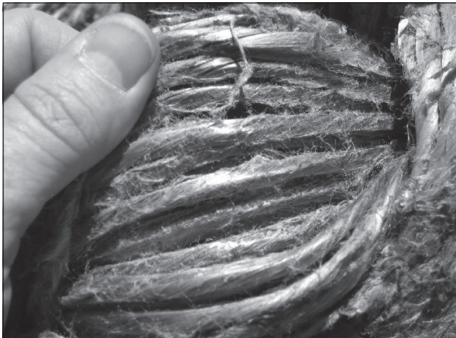
Figure 11: Example of heavy internal abrasion.
